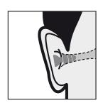
The plug will then be correctly positioned in the ear canal ensuring it offers maximum hearing protection.
